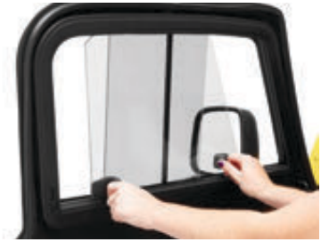
TJ Wrangler Upper Door sliders offer dual sliding glass panels that "click" shut with one hand
