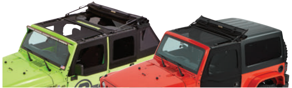
Sunshade securely latches to footman loops
