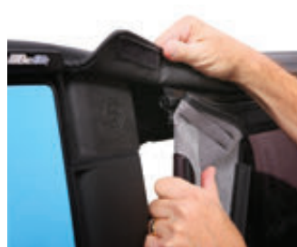
Zipperless technology used in key areas to improve fit and installation
